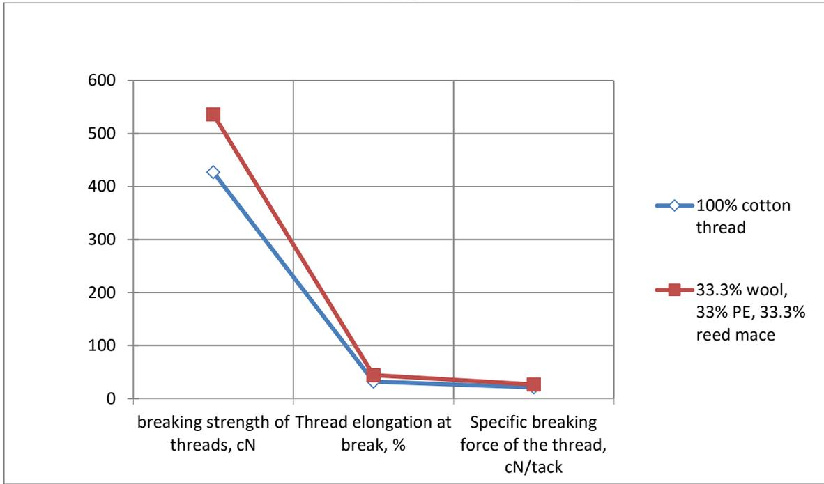
**Fig. 1. Physical and mechanical properties of yarn**
