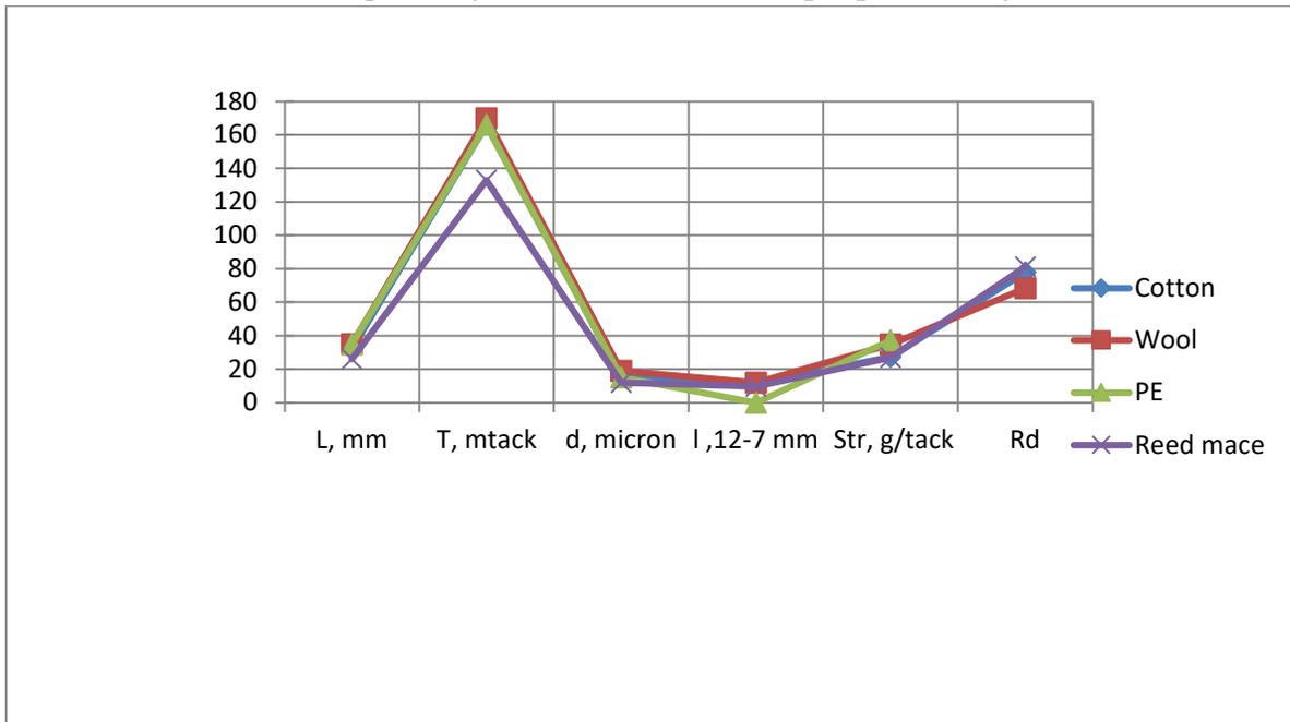
L is fiber length, mm; T is the linear density of the fiber, mtack; d is the fiber diameter, micron; l is short wave index, 12-7 mm; S is the specific tensile strength of the fiber, g/tack; Rd is beam reflectance
