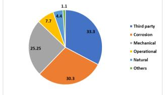
Fig. 1 Percentage of causes of damage in oil and gas pipeline [4]
