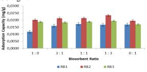
Fig. 1 Adsorption capacity of Zn by mixture S. cinereum and Rhizobacteria in the modified tea bag
