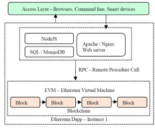
Fig. 6 An overview of the system architecture
