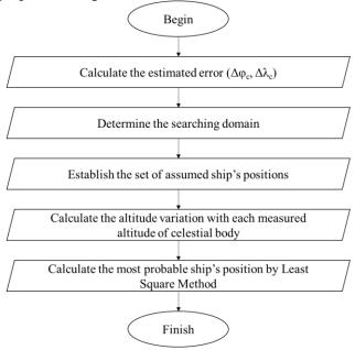
Fig. 7 Flow chart of ship positioning by the celestial altitude difference based on the Least Squares Method
