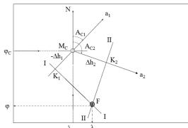
Fig. 5 Ship positioning by plotting the COP on nautical chart
