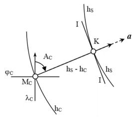
Fig. 4 The circle of position on the nautical chart
