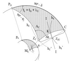
Assumed that the ship's true position is  $M_0(\varphi_0, \lambda_0)$  at the same time, then measure and adjust the true altitude  $h_s$  to the celestial body C and the true zenith distance  $Z_s = 90^0 - h_s$ . The ship's true position will be at the circle of equal altitude  $h_s h'_s$  with the center as the position of celestial body C, radius as the zenith distance  $Z_s = 90^0 - h_s$ .
