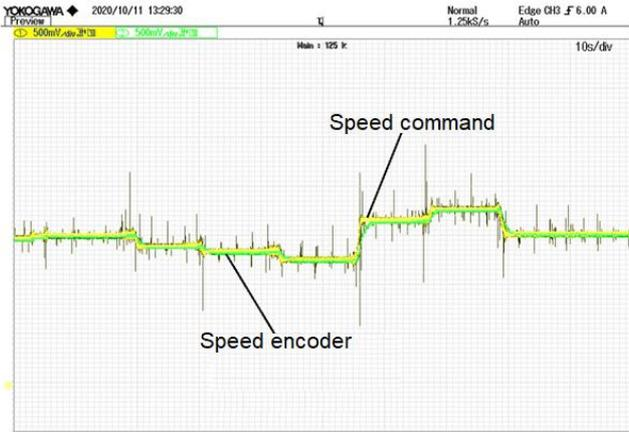
Fig. 7 Step speed command signal comparison with the speed encoder
