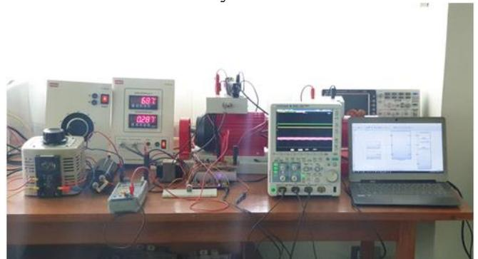
Fig. 6 The response of the prototype for the DC motor control
