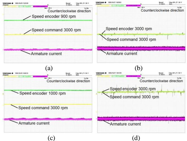
Fig. 10 Speed control of DC motor in three-quadrant
