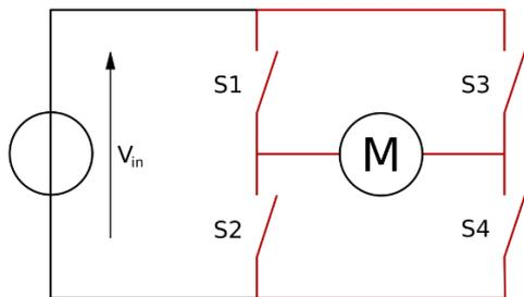
Fig. 2 The structure of the H-bridge drive mechanism with the motor as a load
