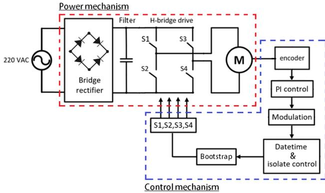
Fig. 1 Mechanism diagram of the H-bridge bootstrap topology
