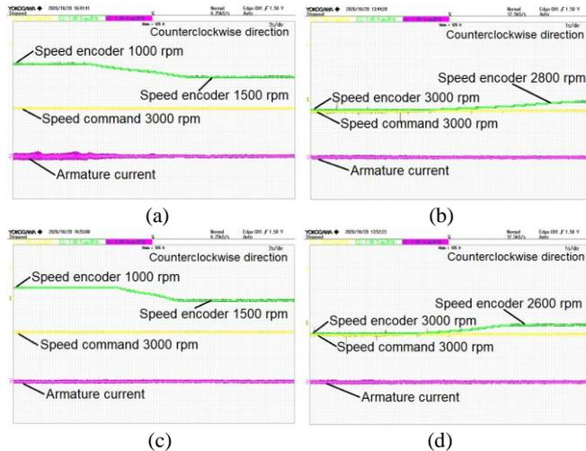
Fig. 11 Speed control of DC motor in four-quadrant
