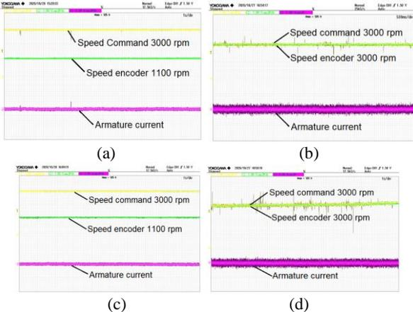
Fig. 8 Speed control of DC motor in one-quadrant
