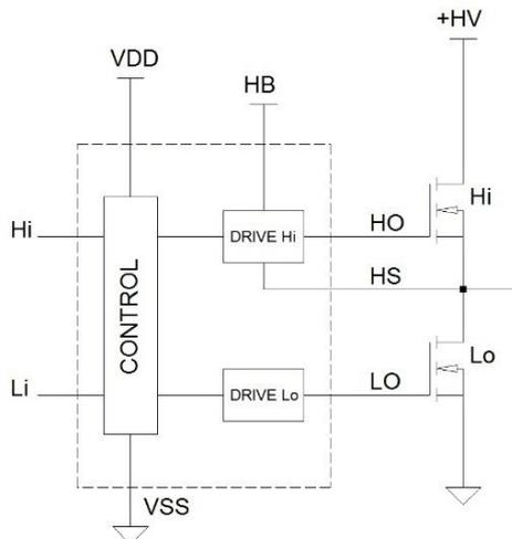
Fig. 4 Basic IC High-Side Driver circuit using Bootstrap technique
