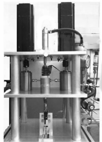
图6 电控液压全可变气门驱动系统试验台架 Fig.6 Experiment of the proposed system
